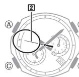
**3. The receive operation is complete when the **2 Second Hand** moves to **Y** (**YES**) or **N** (**NO**) for about five seconds, and then resumes regular timekeeping.**
