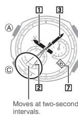
You can get an idea of the watch's power level by observing the movement of the **[2] Second Hand** in the Timekeeping Mode.
